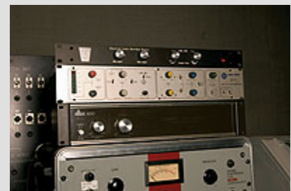
Some of the more unusual rackmounting gear at Electrical Audio: from top, custom-built mid/sides matrix, Klark-Tech DN34 'Analogue Time Processor', Dbx 500 subharmonic generator and Skibbe 5-9C compressor.
